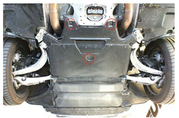
STEP 2 Remove the two plastic rivets that are circled, use a flathead screwdriver or panel remover tool.
